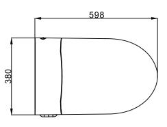
All drawings contain the necessary measurements which are subject to standard tolerances. They are stated in mm and are non-binding. Exact measurements, in particular for customized installation scenarios, can only be taken from the fished ceramic piece.
